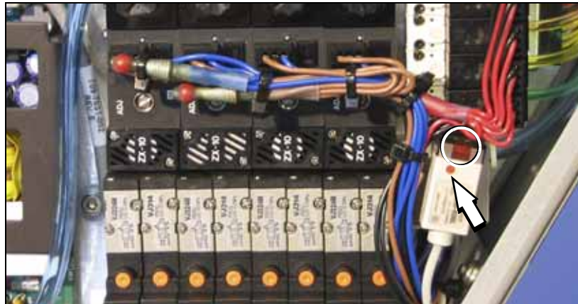
Figure 14—Adjusting the Low Pressure Sensor on the Pneumatic Module. The arrow points to the adjustment screw. The LED is circled.
