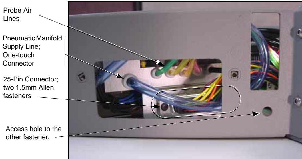
Figure 12—Location of the Pneumatic Manifold Supply Line and Wiring Connector
