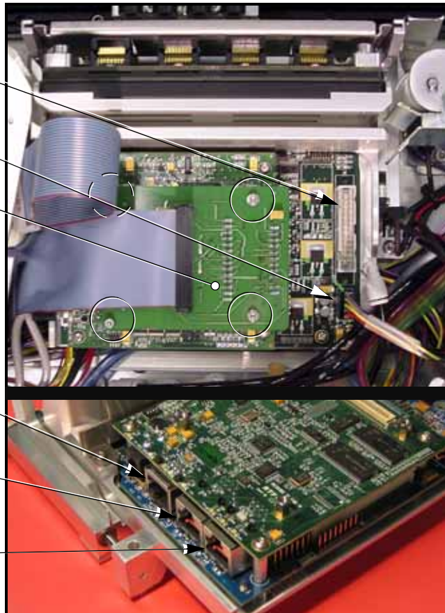
Figure 35— Cable Connectors and PCMCIA-PCB fasteners on FCIII.
