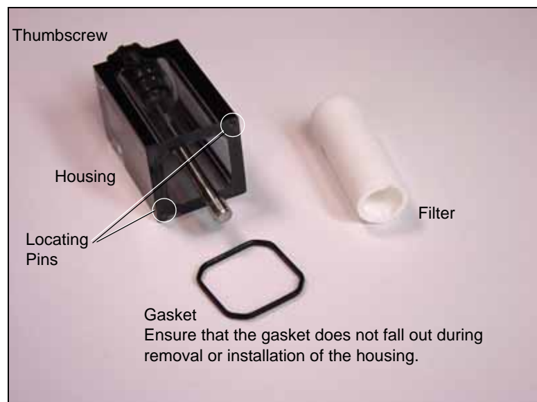
Figure S-11—Vacuum Filter Components
