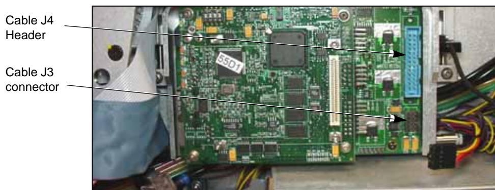
Figure S-38—Cable J3 and Header J4 Locations
