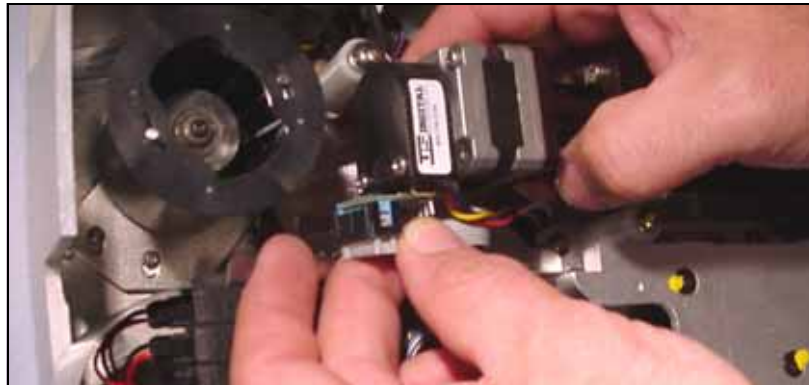
Figure S-45—Disconnecting the Ribbon Cable from the Encoder.
