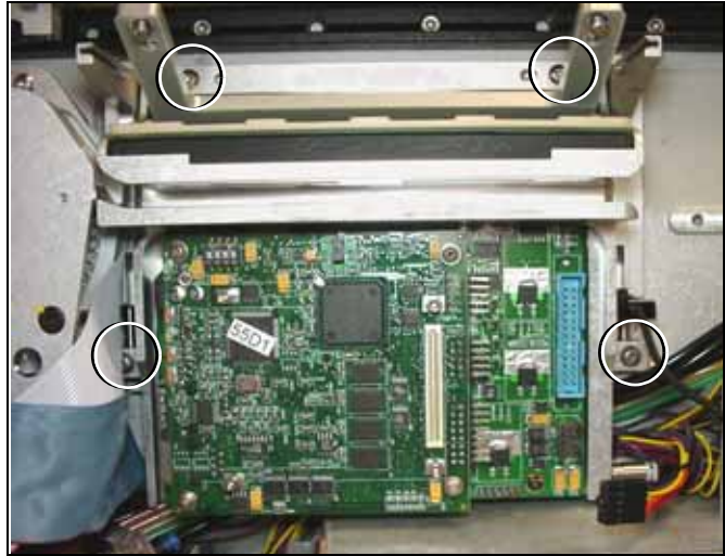
Figure S-39—Location of Programmer Screws
