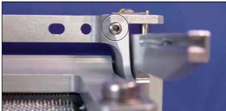
Figure S-41—Programmer Module Alignment Screws (the Left Screw is not shown)
