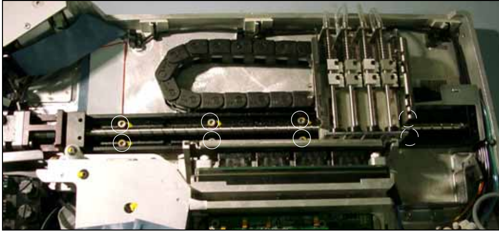
Figure S-44—Linear Stage Screw Locations. (Two are hidden by the head.)
