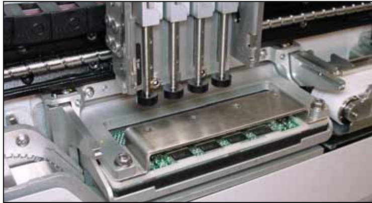
Figure S-40—The Programmer Module Alignment Tool Installed on the Programmer
