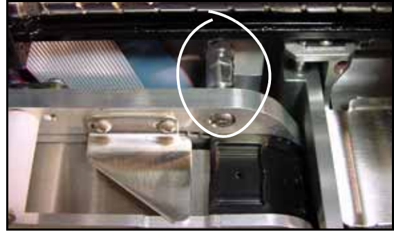
Figure S-8—Some Tape-In Modules have an Adjustable Standoff for setting the Alignment with the Probes. The wrench flats and Locknut identify the Adjustment Stud from a non-adjustable Standoff.
