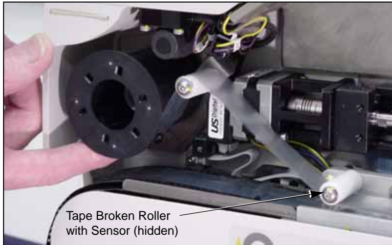
Figure S-16—Cover Tape Tensioning the Tape Broken Sensor
