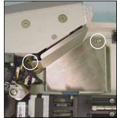
Figure S-27—Ribbon Cable Guard Screw Locations
