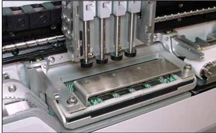
Figure P-40—The Programmer Module Alignment Tool Installed on the Programmer
