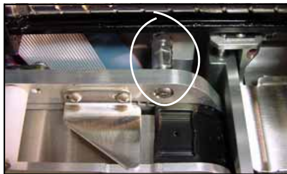
Figure P-9—Some Tape-In Modules have an Adjustable Standoff for setting the Alignment with the Probes. The wrench flats and Locknut identify the Adjustment Stud from a non-adjustable Standoff.
