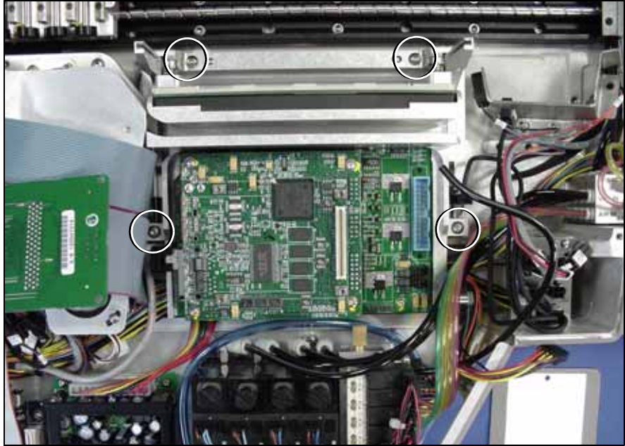
Figure P-39—Location of Programmer Screws
