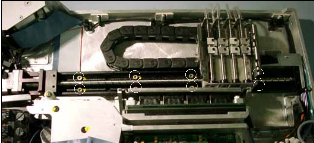
Figure P-44—Linear Stage Screw Locations. (Two are hidden by the head.)
