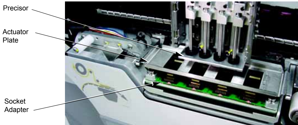
Figure P-49—Precisor, Actuator, and Socket Adapter Locations
