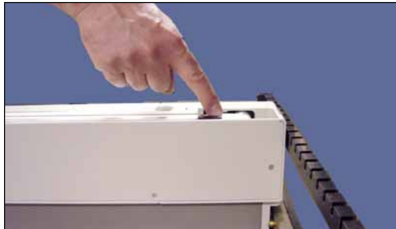
Figure P-22—Testing the End-of-Belt Sensor (The Conveyor Cover need not be removed.)
