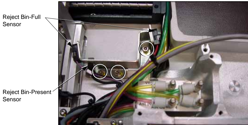
Figure F-28—Reject Bin Sensors and Bracket Screw Locations.
