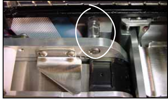
Figure F-10—Some Tape-In Modules have an Adjustable Standoff for setting the Alignment with the Probes. The wrench flats and Locknut identify the Adjustment Stud from a non-adjustable Standoff.
