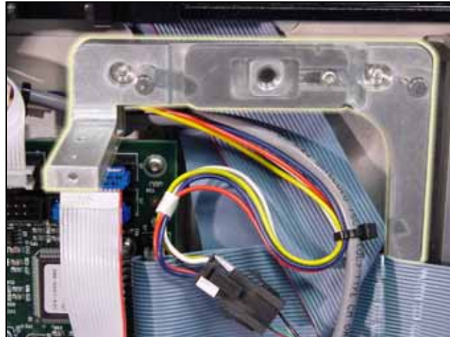
Figure A-6—Adjustable Tape-In Module Base
