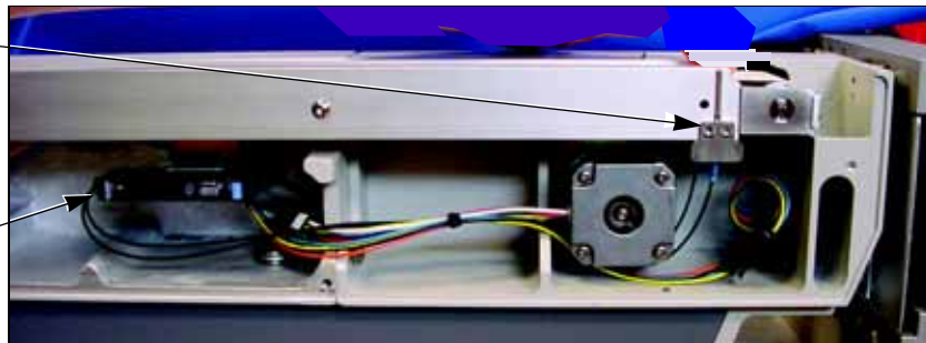
Figure A-24—Reteaching the End-of-Belt Sensor [Universal Shown]
