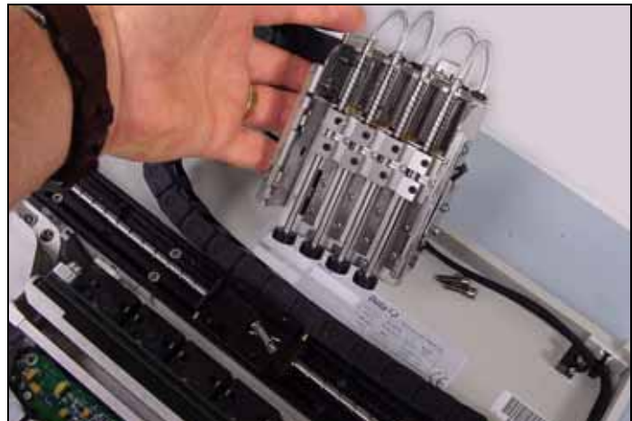
Figure A-35—The PNP Head Partially Removed
