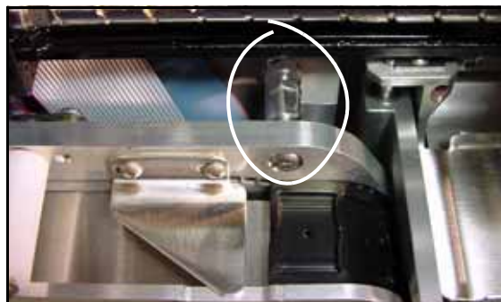
Figure A-9—Some Tape-In Modules have an Adjustable Standoff for setting the Alignment with the Probes. The wrench flats and Locknut identify the Adjustment Stud from a non-adjustable Standoff.
