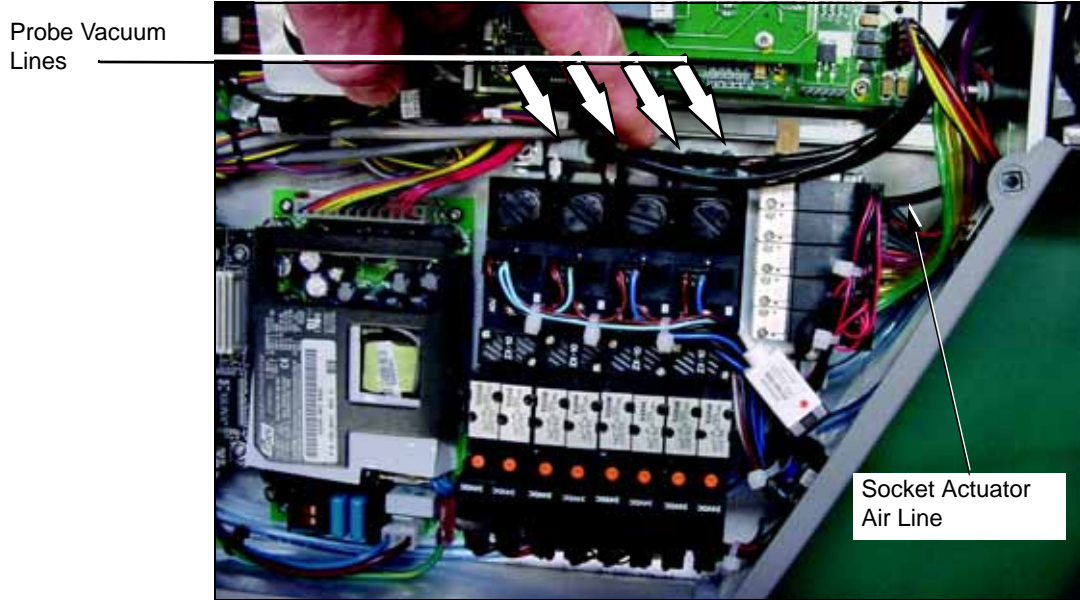
Figure A-14—Location of Vacuum and Air Lines
