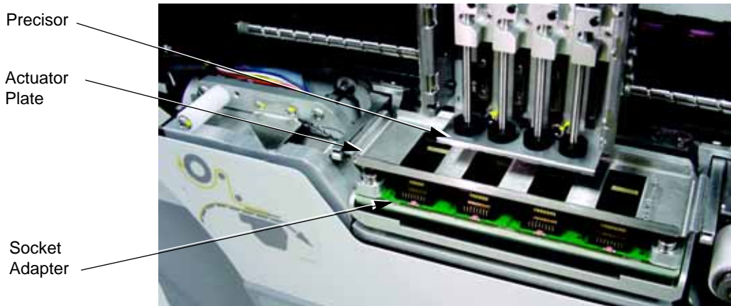
Figure A-50—Precisor, Actuator, and Socket Adapter Locations
