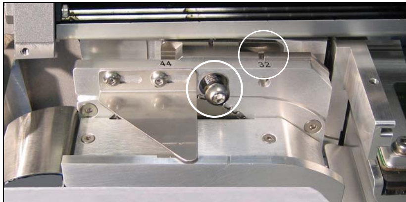
Figure 3-12—XLF Models ONLY, have a 32/44 mm Tape-In Module. The notch currently indicates 32 mm. The Position Locking Screw is loosened. The 32 mm Front Track is not shown.
