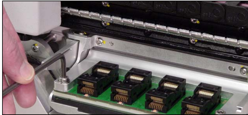
Figure 3-3—Removing the Screws Securing the Socket Adapter
