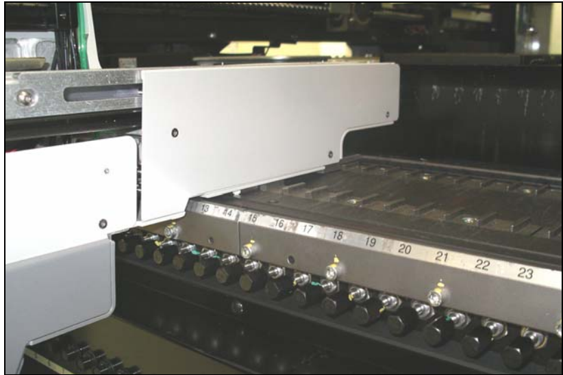
Figure 2-15—RoadRunner/Panasonic mounted on the Feeder Bank.
