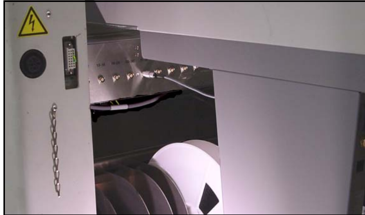
Figure 2-31—[Siemens] Communications Cable Plugged into the SIPLACE Feeder Table
