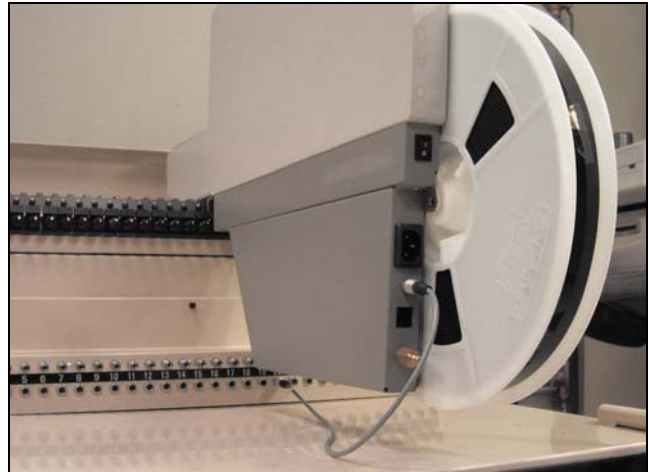
Figure 2-10—The RoadRunner mounted onto a Multi Feeder Unit (MFU)
