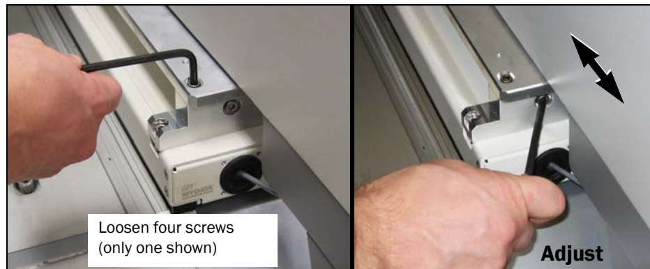
Figure 2-8—Adjusting the pick point.
