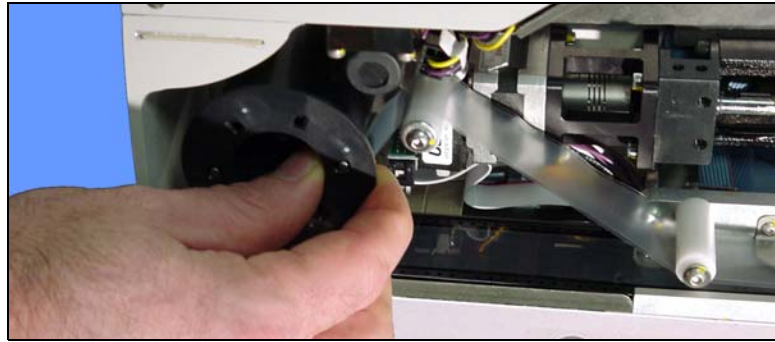
Figure 3-16—Attaching the Cover Tape to the Take-up Reel on standard RoadRunners [Siemens Model Shown].
