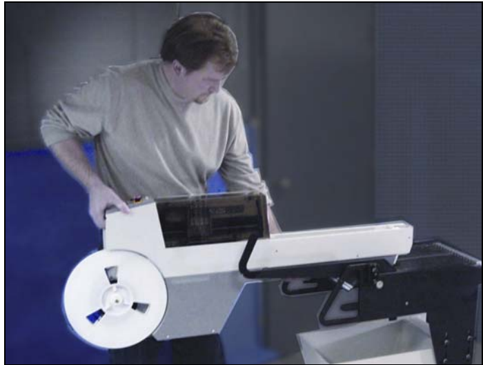
Figure 2-26—Mounting RoadRunner onto a Feeder Bank Changer.
