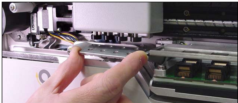
Figure 3-5—Removing the Precisor [Siemens Model Shown]
