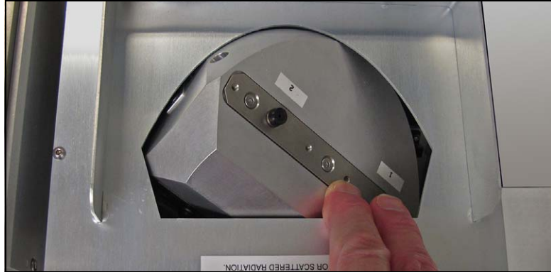
Figure 26: The Laser rotor can be rotated by hand when the motor is disabled (or the machine power is OFF).
