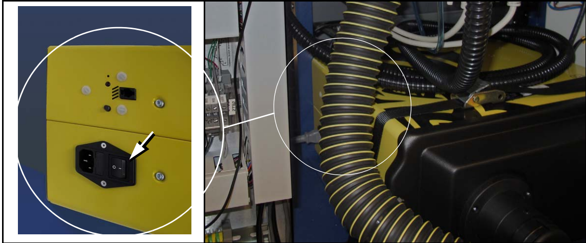
Figure 40: Fume Extractor Power Switch (hidden behind hose).
