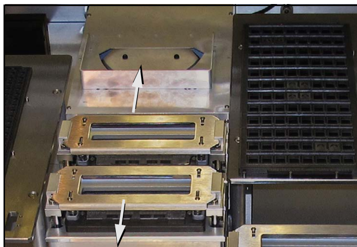
Figure 16: Remove the Actuator Plate by sliding it out from the bracket in either direction; sockets must be closed (up position). If the
