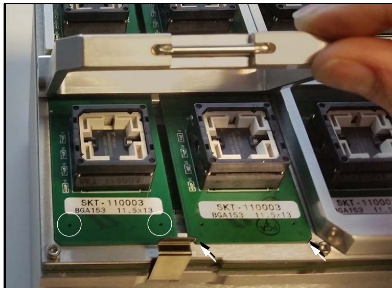
Figure 21: One clamp open with Socket Adapters. Two of the alignment holes are circled. The two back alignment holes are not visible in this view. Chamfers are to the front (arrows).
