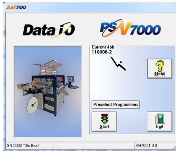
Figure 33: The AH700 Main window opens with a job loaded and the job name displayed (arrow).
