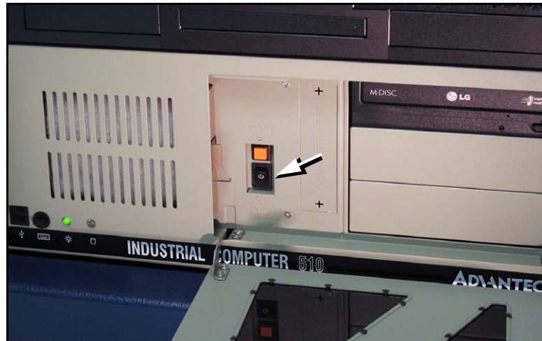
Figure 13: The 3D Coplanarity Computer is below the Handler Computer on the left side of the machine. Power Switch (arrow).
