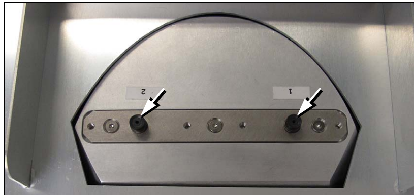
Figure 25: A 1.5 mm hex key fits into the center of the each laser tip to unscrew it.
