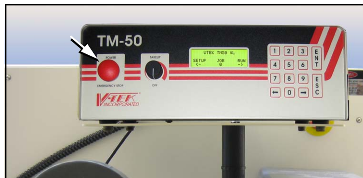
Figure 4-30: Tape Output Module Controller. The arrow points to the Power On/Off button which is also the Emergency-Stop (for the Tape-Out Module only!).
