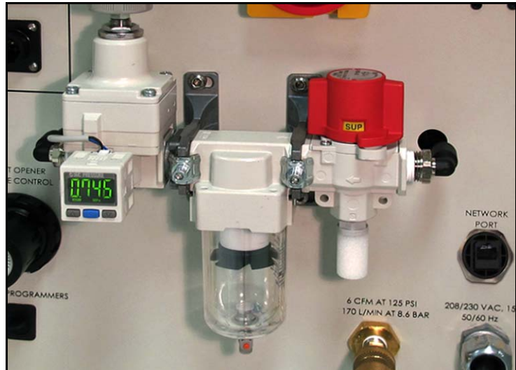
Figure 4-1: The input air regulator/filter on the Power Panel (on the left side of the machine). When the lock rings on the valve line up, the air supply to the PSV7000 Machine is OFF.
