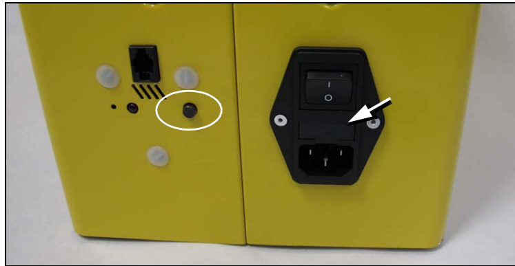
Figure 4-21: Tiger Fume Extractor power switch, utilities, reset button (circled), and fuse location (arrow).
