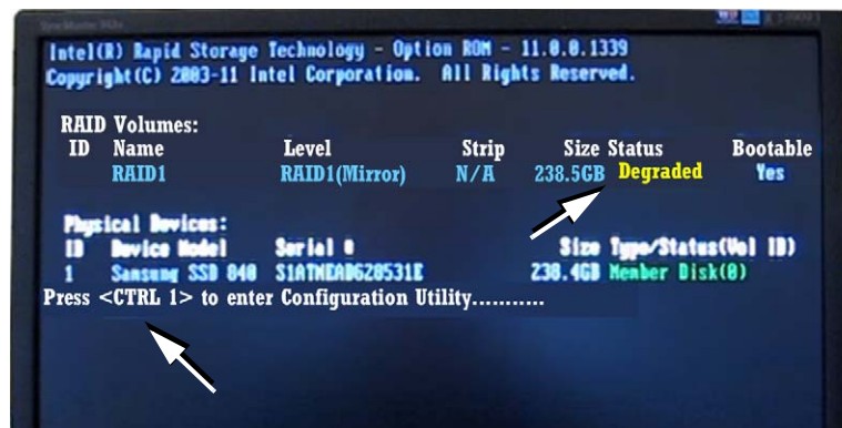
Figure 4-28: This message, DEGRADED , will display for about seven seconds at startup if a Handler drive has failed.
