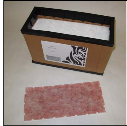
Figure 4-24: The Pre-Filter is removed from the Main Filter.
