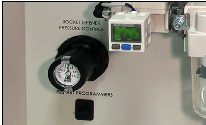
Figure 4-2: The Socket Opener Pressure Control knob with built-in gauge on the Power Panel.
