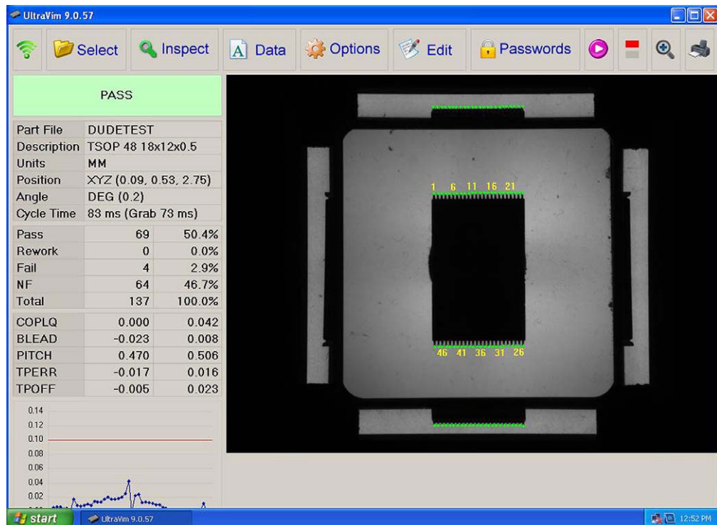
Figure 3-19: A good inspection image. The dot at each lead is green.
