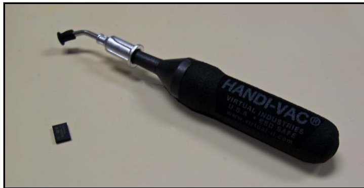
Figure 1-1: A Vacuum Tweezer: Data I/O PN 565-8000-001.
