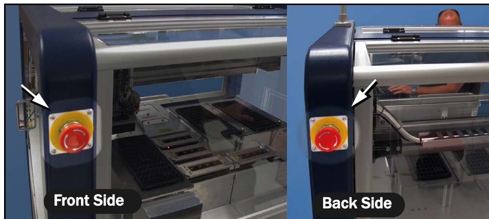
Figure 1-3: Two Emergency Stop (E-Stop) buttons.
