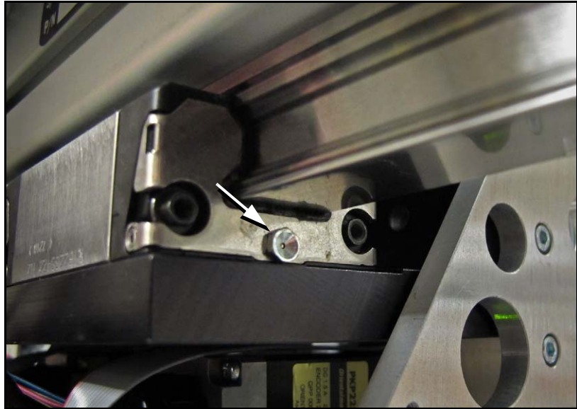
Figure 4-12: Grease fitting on the X-axis guide, shown.
