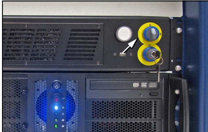
Figure 3-12: The Laser PC Enable Selector (arrow) and the Key Selector.
