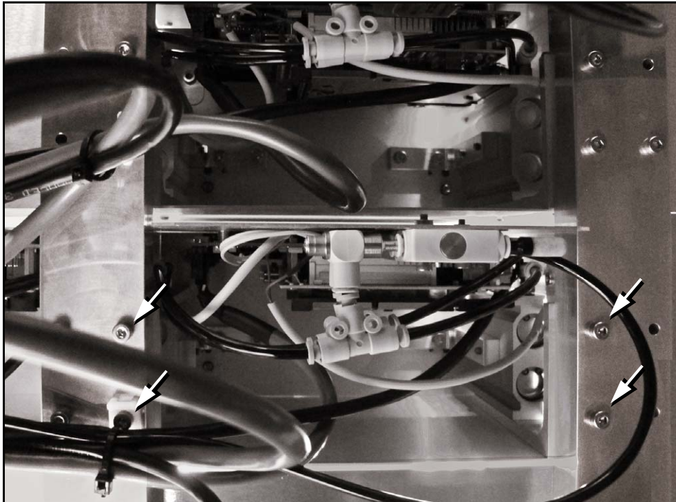
Figure 4-20: Inside the machine looking up at the programmers. There are four attachment screws (arrows) per programmer.
