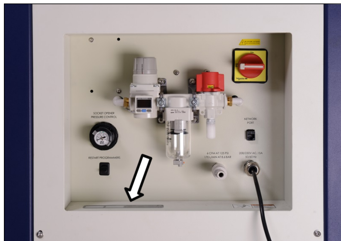
Figure 10: Power Panel (Facilities Panel) on the back of the machine. The Serial Number is there, also (arrow).
