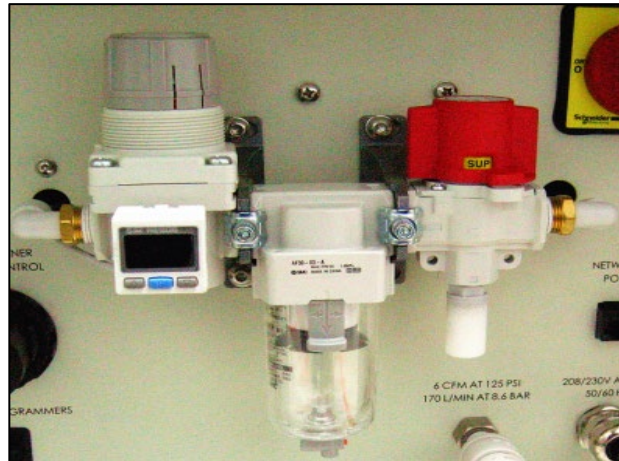
Figure 57: Input air regulator/filter on the Power Panel (on the left side of the machine). When the lock rings on the valve line up, the air supply to the PSV5000 Machine is OFF.
