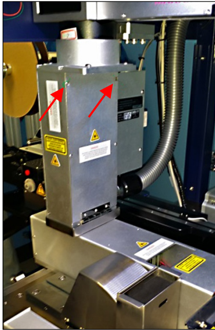
Figure 52: Fasteners on the laser inspection door (arrows).
