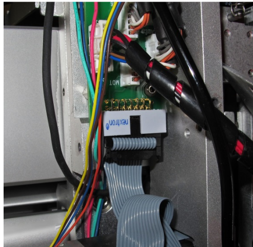
Figure 71: Unplug the ribbon cable from the back.
