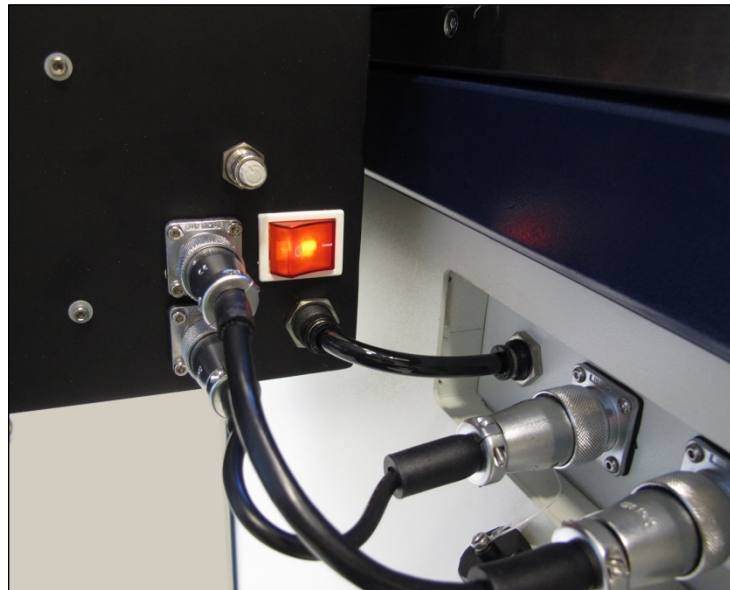
Figure 24: Connection for the Tray Feeder: air, electrical and signal (left to right).
