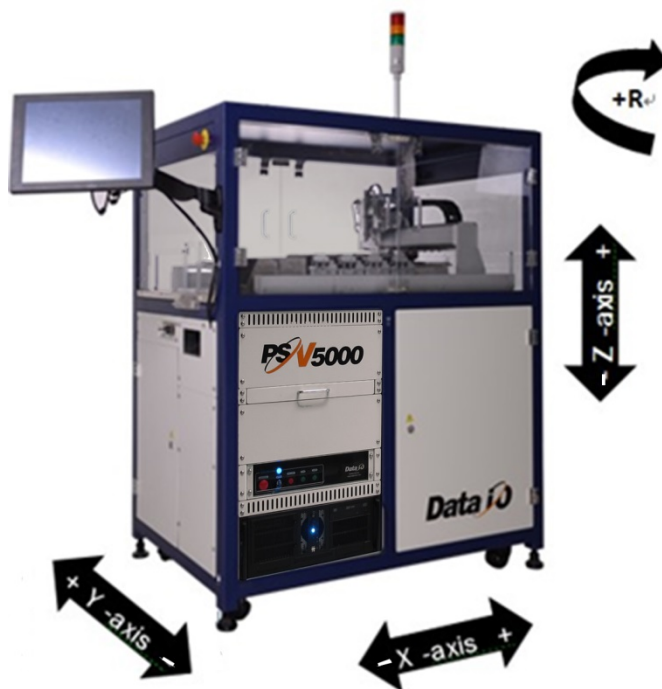
Figure 5: These axes describe motion direction on the PSV5000. The X-Y coordinate 0, 0 is at the left front corner.
