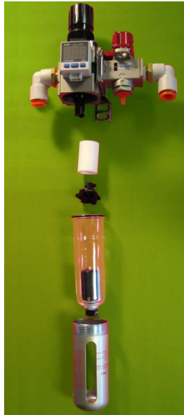
Figure 64: Replacing the Air Filter/Regulator.
