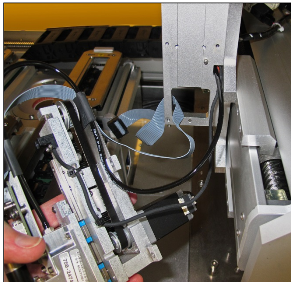
Figure 74: Probe Assembly is removed with the tubing and wires still through the head mount.
