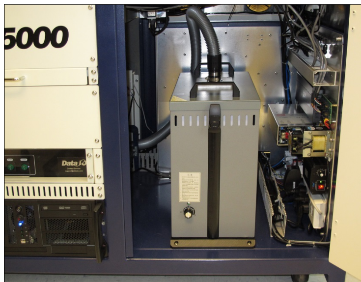
Figure 77: The Fume Extractor inside the front of the PSV5000.
