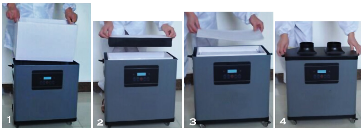
Figure 78: These four steps show filter replacement. Refer to the Fume Extractor Operation Manual.
