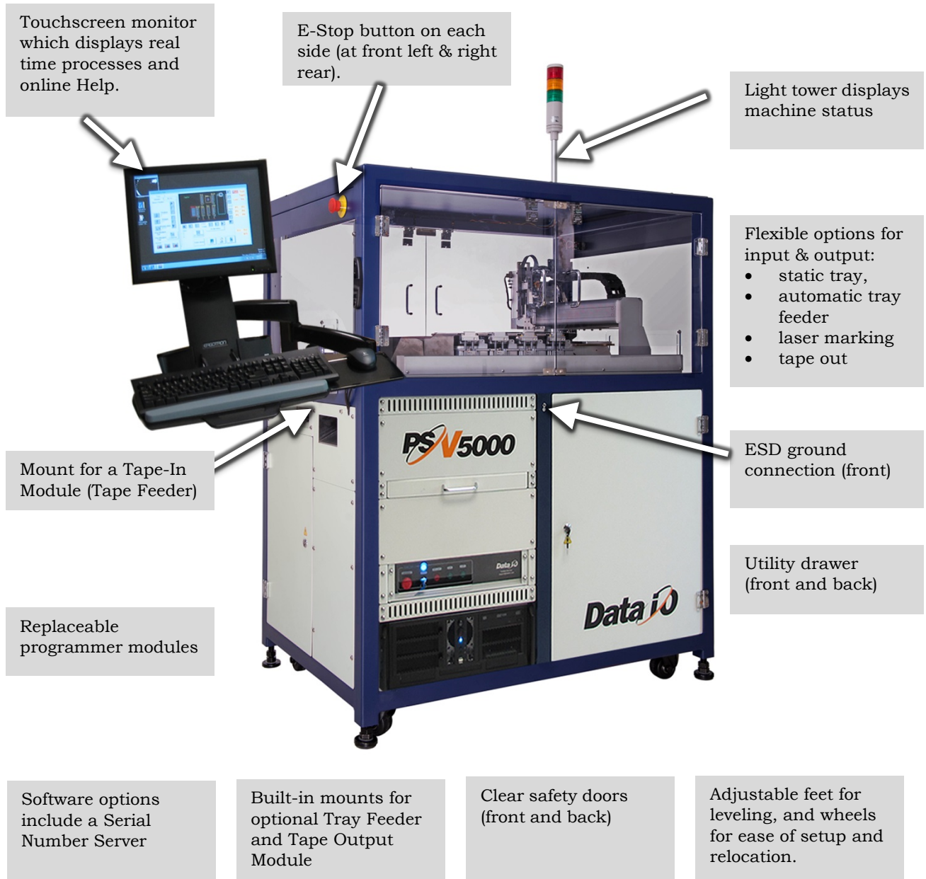
Figure 1: Features of PSV5000. For a more detailed image with components labeled, see the Operator's Manual. For component descriptions see Component Descriptions on page19.
