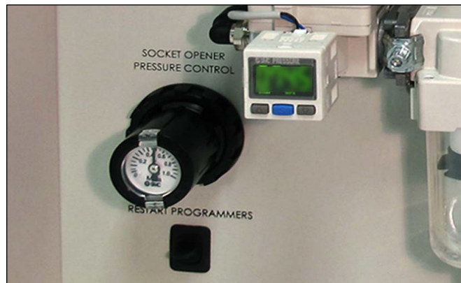
Figure 58: The Socket Opener Pressure Control knob with built-in gauge on the Power Panel.
