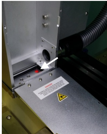
Figure 54: If laser is activated, there will be a red spot at location of the arrow.
