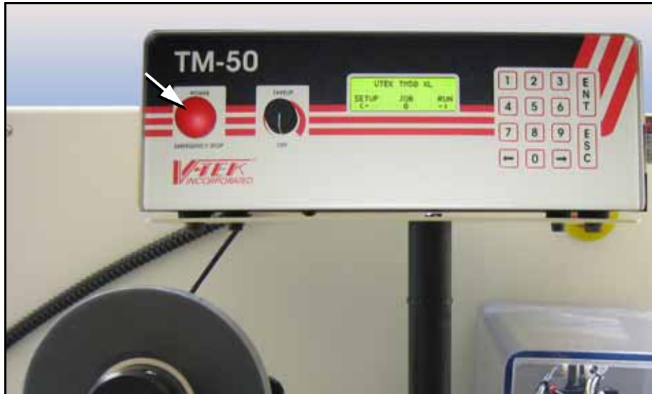
Figure 4-61: Tape Output Module Controller. The arrow points to the Power On/Off button which is also the Emergency-Stop.
