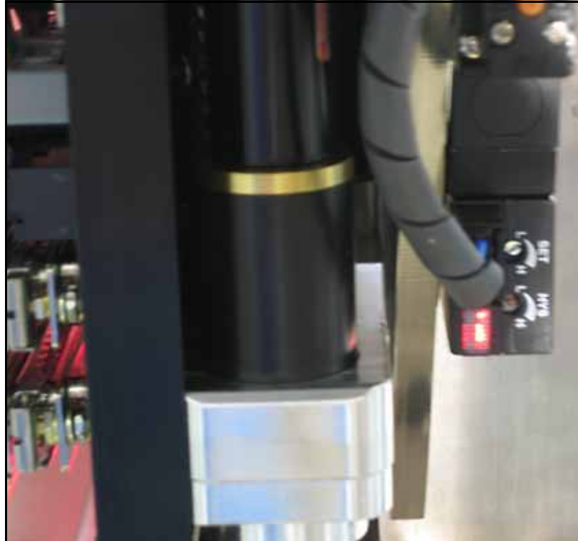
Figure 4-16: The PNP Probe vacuum generator adjustments. Your PNP head may not look like this.)
