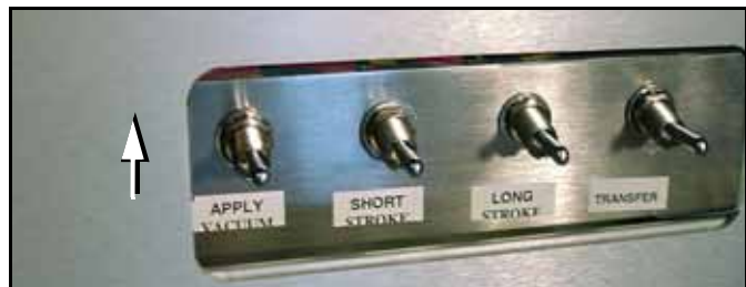
Figure 4-19: Apply Vacuum switch: UP is on.
