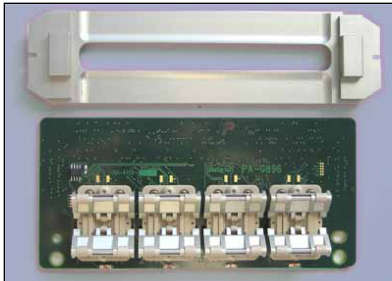
Figure 3-4: Special Actuation Plate for HIC Adapters.
