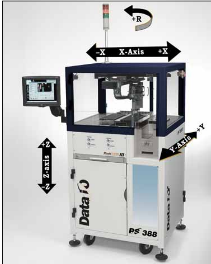
Figure 1-1: These axes are used throughout this manual to describe motion or direction of components of the PS System. They are the same for all PS Machines. (PS388 shown.)
