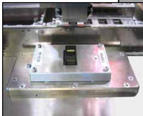
An Optima Programmer installed, with a Socket Adapter on it.
