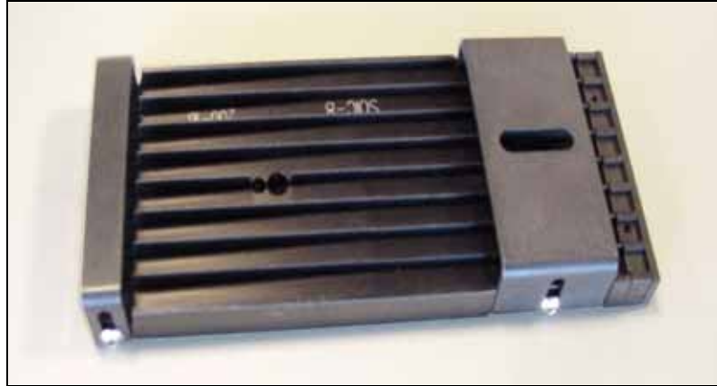
Figure 2-14: Output tube unloader platform.
