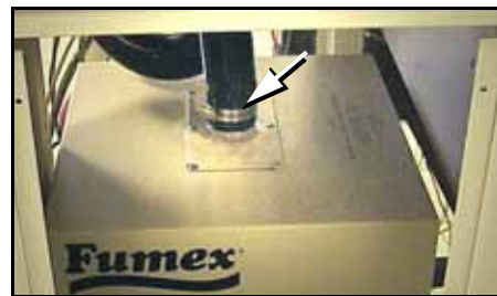
Figure 4-41: The Vacuum hose clamp.
