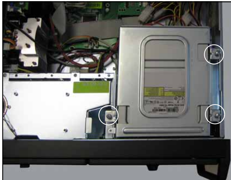
Figure 4-60: Three Phillips screws (circled) secure the bracket holding all the hard drives that are accessible from the front of the PS Machine. Your PC Box and bracket may be different depending on manufacture date.
