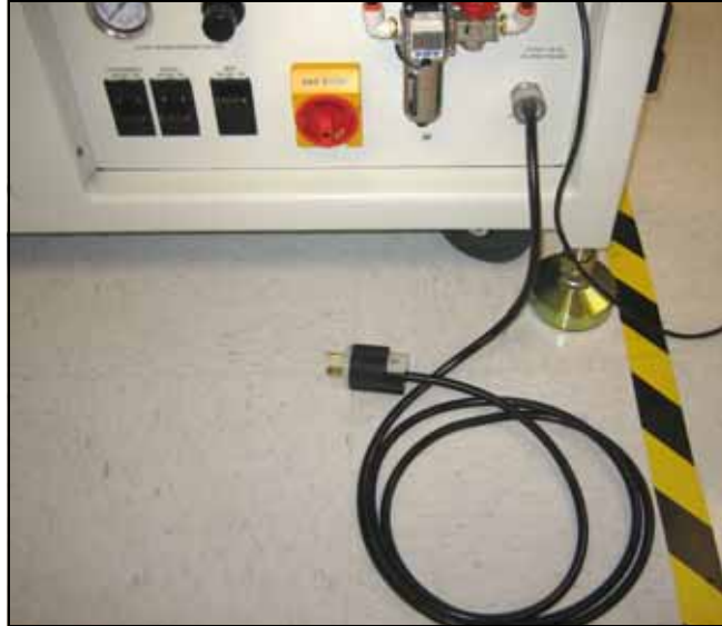
Figure 2-2: Electrical power cable and plug. The machine end of the cable is not removable.
