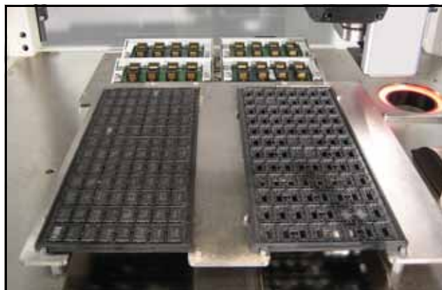
Figure 1-6: Static tray mount on PS288.
