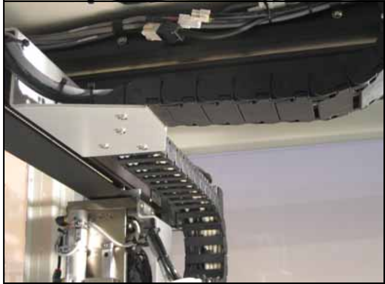
Figure 4-25: The two cable carriers meet at a bracket at the back of the PS System. There are two screws for each carrier end. View looking upward from the back of the machine.
