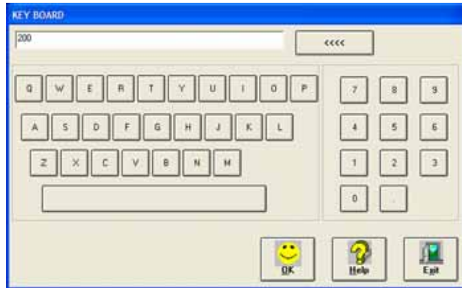
Figure 3-22: The Keyboard dialog opens after clicking in the Pass Limit field. The <<<< button erases the right-most digit. Exit cancels any changes.
