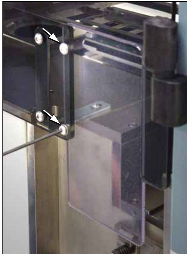
Figure 2-15: Two screws holding the small safety shield. [PS588 shown.]
