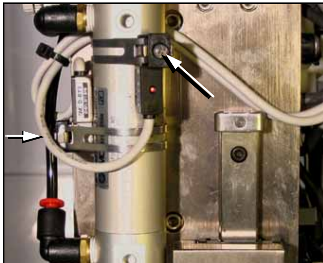
Figure 4-2: Cylinder Sensors for determining socket actuator positions; viewed from back of PNP head. The long arrow points to the adjustment screw for the Up position sensor and the short arrow for the down sensor (screw partially hidden). Sensors may be radially oriented differently on the cylinder.
