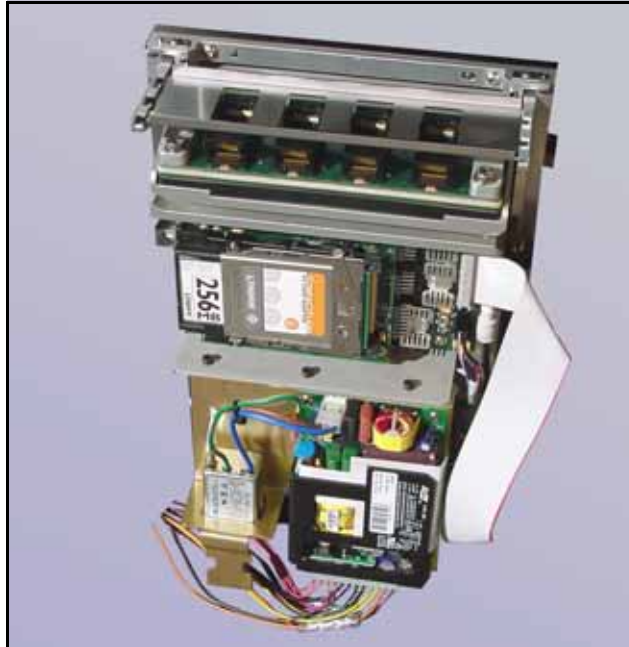
Figure 1-5: A FlashCORE Programmer with a Socket Adapter and Actuator Plate installed on it.
