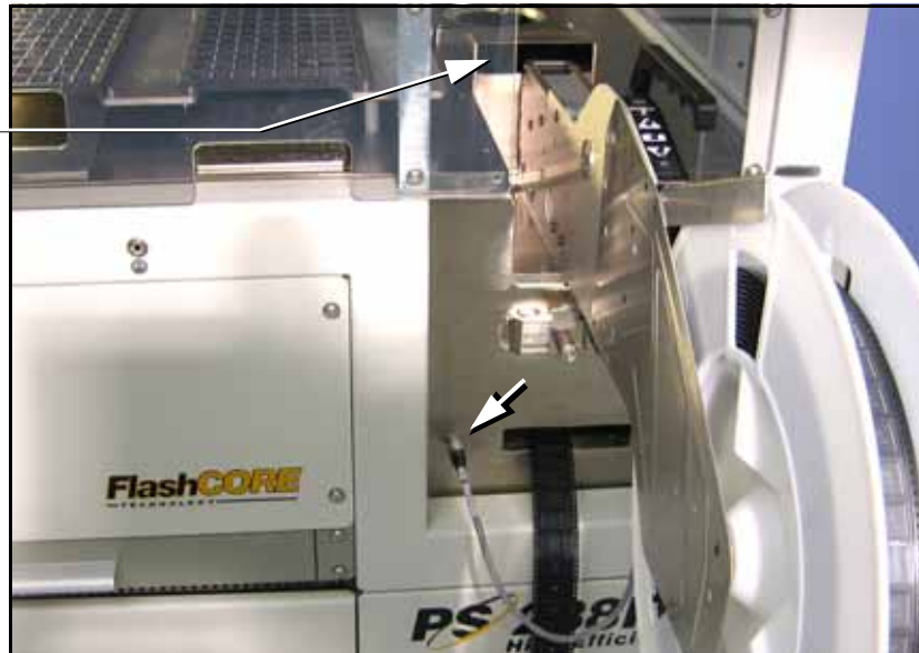
Figure 2-18: The Tape-Input cable is plugged into the front of the PS Machine. (PS288 shown.)
