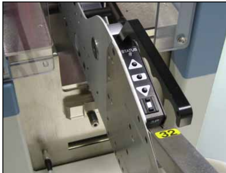
Figure 3-42: A chip feeder mounted on a PS388.
