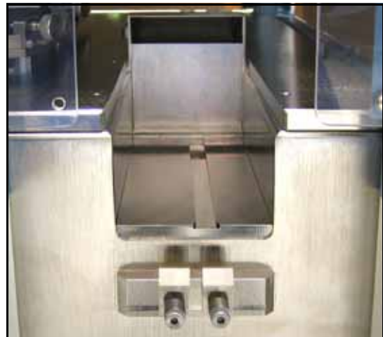
Figure 2-16: The channel and spring clamps on the PS Machine.
