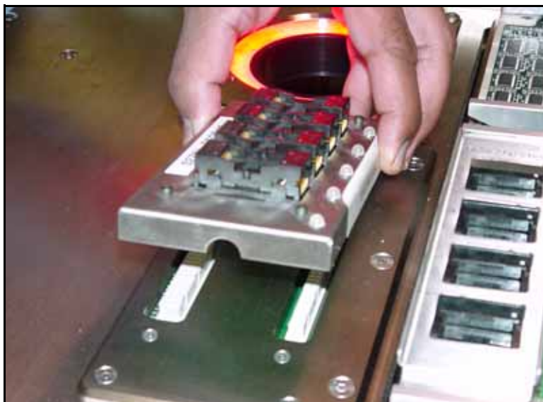
Figure 3-7: Align Socket Adapter and programmer base connectors
