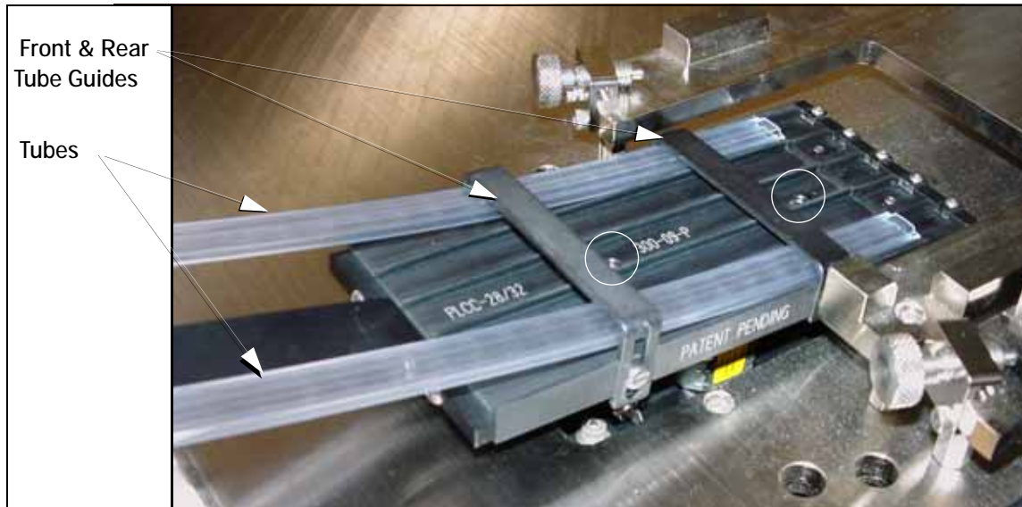
Figure 2-13: Adjust the front and rear tube guides with two empty tubes installed. Platform mounting screws are circled. Tray mounts (with thumb screws) need not be removed from the work surface.
