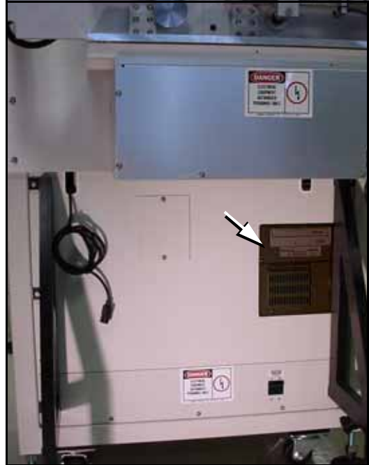
Figure 4-44: The location of Laser Computer filter on the back of the Laser Marker frame. (Some models only.)
