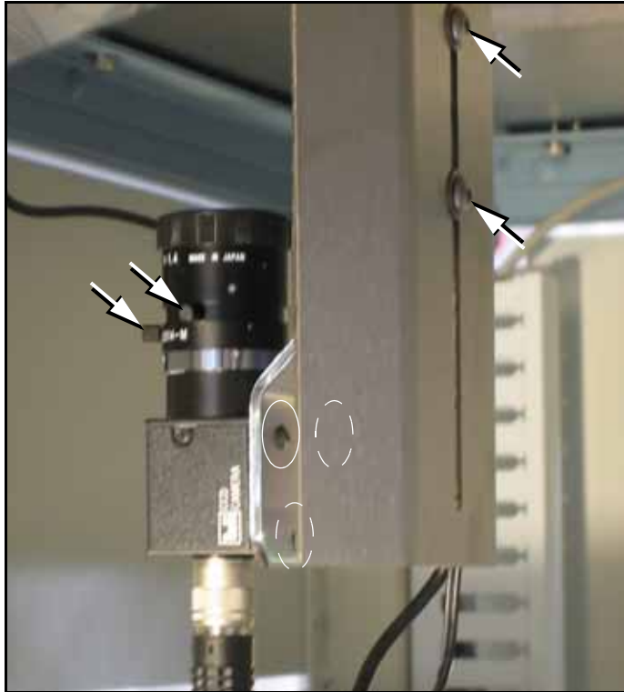
Figure 4-47: Camera mounting screws and focus ring knobs. Dashed ovals indicate screws hidden in this view.
