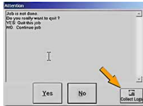
Figure 4-55: The Collect Logs button starts the Collect PS Logs Application in Auto Mode.
