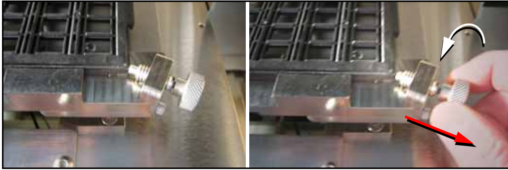
Figure 2-5: To remove a tray, unscrew the thumb screw and lift the tray out. A second method is NOT RECOMMENDED: pulling the thumb screw back and holding it away from the tray while lifting the tray out; if the thumb screw is released too soon, devices may be knocked out of the tray.
