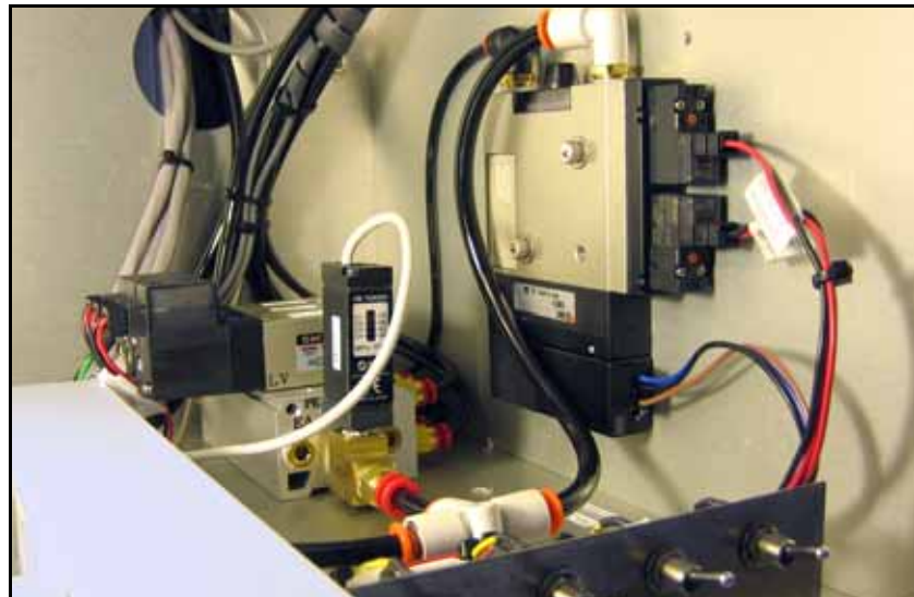
Figure 4-14: A Vacuum Generator on the TM50 Taping Module. The front panel has been removed with a 1/8 in. hex key (six SHCS).
