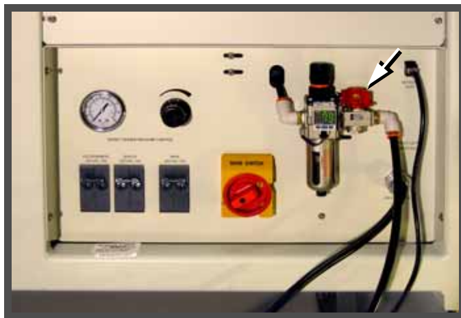
Figure 3-17: Main air valve on the back of the machine.
