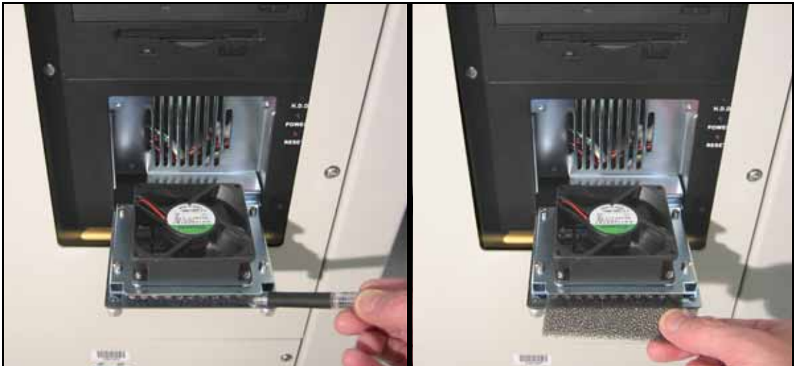
Figure 4-45: After opening the Laser Marker Computer filter cover, drag the filter out with a pen or pencil. (Early filter covers are not hinged.)
