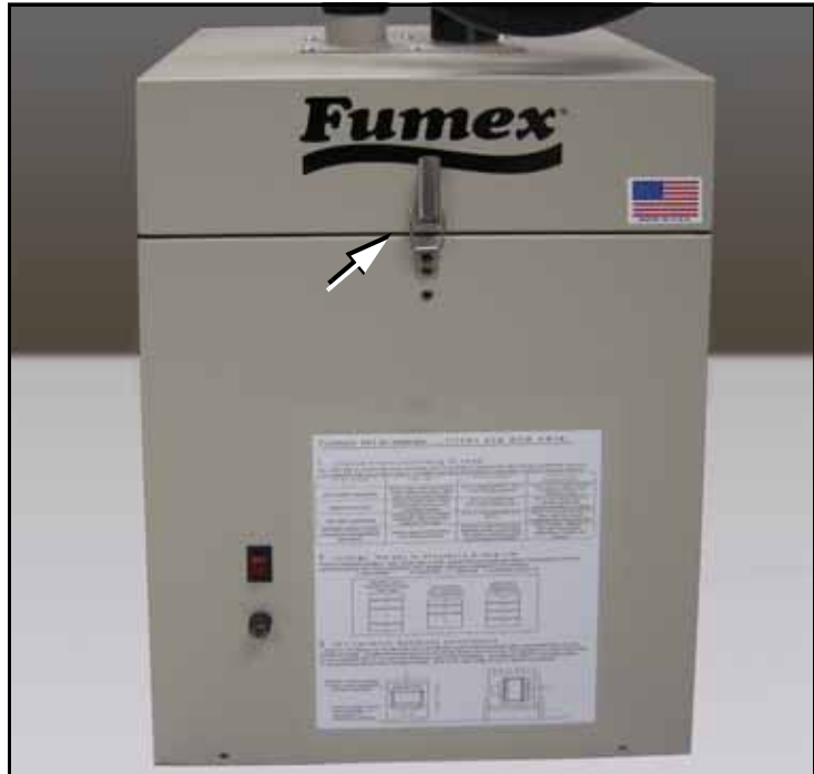
Figure 4-42: One of the spring clips securing the extractor top. Also, the Fumex care label.
